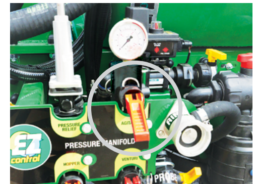
Open the 'Agitator' valve (located on the Pressure Manifold) to ensure chemical agitation in the Main tank.
