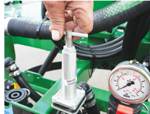
Pressure Relief Valve located on the pressure manifold.
