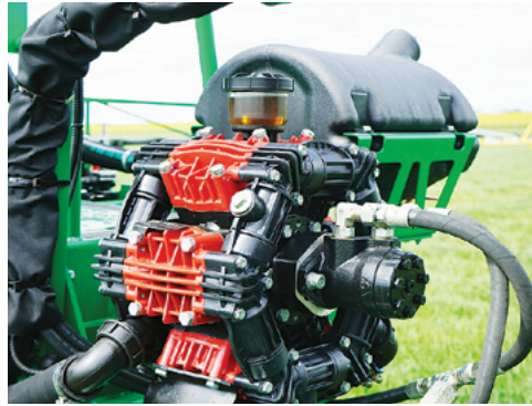
Check diaphragm pump oil level (if fitted).
