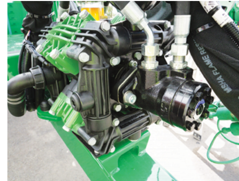
Hydraulically driven diaphragm pump.
