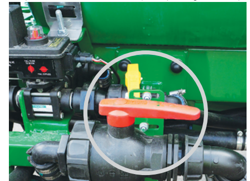
Turn the Three-way Red Handle ball valve (top of the suction filter) to draw from the Rinse tank (arrow pointing rearwards).
