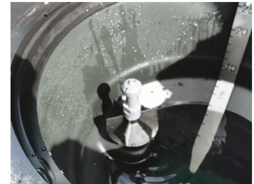
Hopper Drum Rinse Nozzle.
