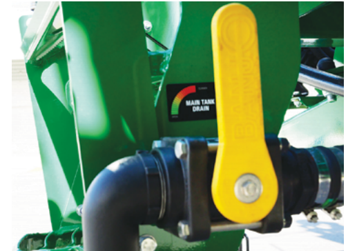
After rinsate is drained from the tank, close the 'Main Tank Drain' valve.
