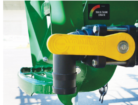
Open the Tank drain ball valve to safely & completely drain the Main Tank.
