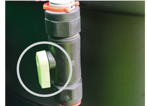
Open the Mixing jet valve on the left hand side of the hopper to start mixing.
