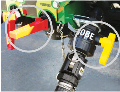
Open the Venturi Valve (Pressure Manifold) and open the Chemical Probe Inlet valve.
