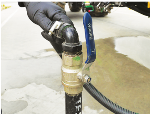
Place the Chemical Probe into the chemical source & open the Probe Valve.
