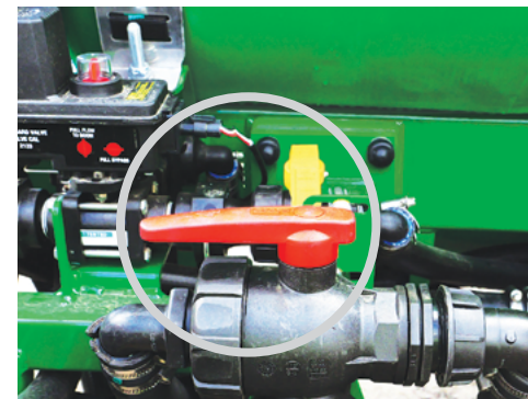
Turn the Three-way Red Handle ball valve (top of the suction filter) to draw from the Main tank (arrow pointing forwards).
