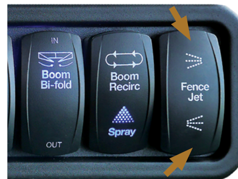
Press the 'Fence Jet' switch to start & stop fenceline nozzle spraying as required.
