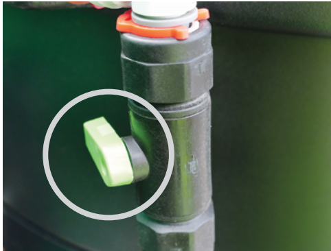
Close the Mixing jet valve on the left hand side of the hopper on completion of transfer.
