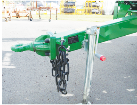
Rotate the jack down, then & wind the handle to raise the hitch until weight is taken off the tractor.
