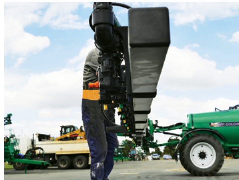
Check Yaw tension by hand on standard booms.
