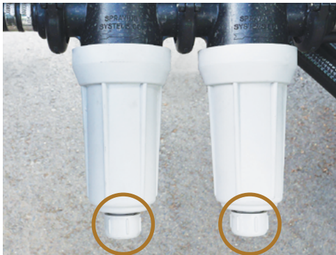
Unscrew and remove the end caps from each filter and allow liquid to drain out.
