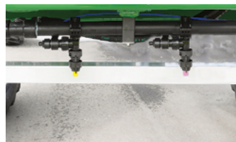
Photo Right: Two nozzles plumbed either side of the centre of the boom - is referred to as Broadacre plumbing.
