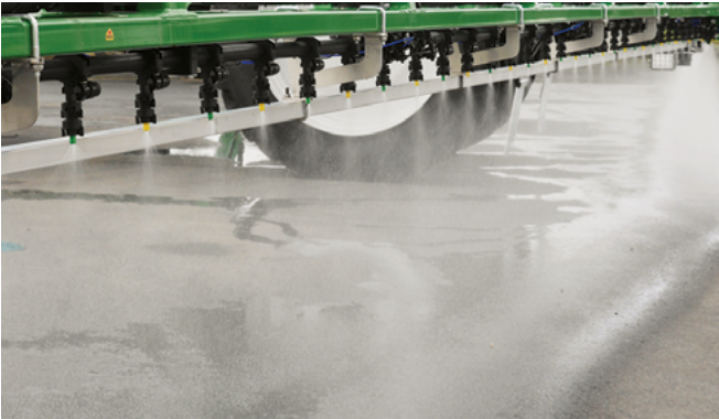
Before measuring nozzle outputs, check for both air & liquid plumbing leaks, kinked or obstructed hoses and good nozzle spray patterns.
