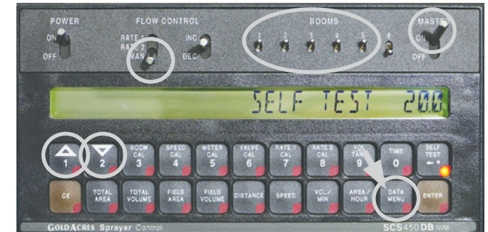
Press 'SELF TEST' touch button & enter normal sprayer operating speed, eg, 20 km/hr. Move BOOMS 'ON/OFF' switches to ON & move the FLOW CONTROL toggle switch to 'MANUAL'. Move 'MASTER ON/OFF' ON to start spraying.
