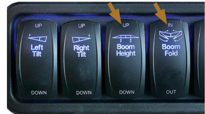
Press the 'Boom Height UP' switch to lift the boom to full height, then the 'Boom Fold IN' to fold in the inner and outer boom sections.
