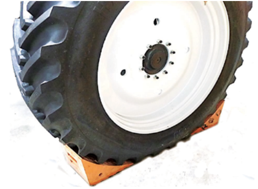
Chock opposite wheel of the sprayer before raising the other wheel off the ground.
