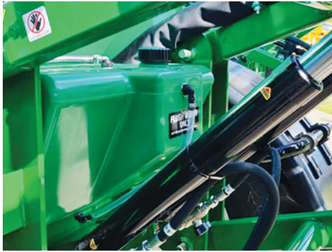
Rinse Tank (200 litres) located at the rear of the sprayer - clean water only for flushing the sprayer.
