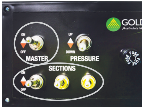
Switch Boom 'SECTIONS' ON and 'MASTER ON' to start boom nozzles spraying.
