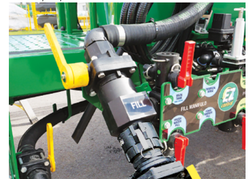
Fully open the '2" Clean Fill Valve' & start the external fill pump to add clean water to the Main tank.
