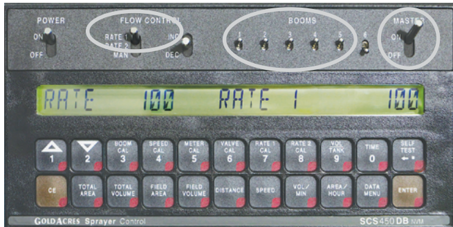
FLOW CONTROL 'RATE 1' toggle switch, 'BOOMS' (sections) ON/OFF toggle switches & boom 'MASTER' ON/OFF toggle switch for the Optional SCS 450 Controller.
