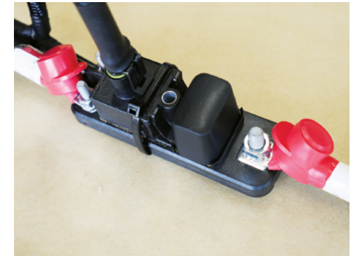
The main power fuse of the Prairie Special electrical system is fitted near the tractor battery.
