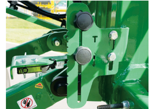
Adjust the Boom Limit Height Setting (located on LHS of the boom centre section) to set minimum boom height.
