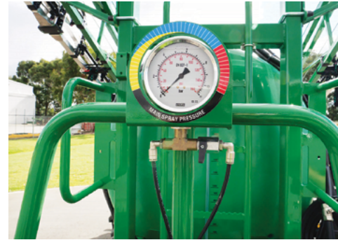
Check hydraulic & spray operating pressures.
