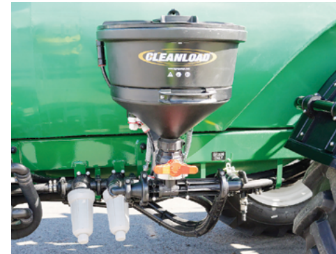
Chemical Induction Hopper in raised/transport position.
