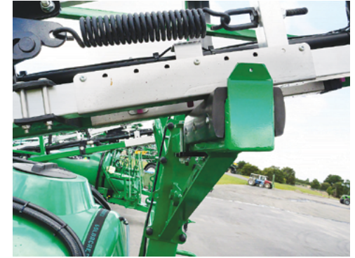
Ensure inside boom & outside boom protector plates are correctly for folding & resting on transport boom rests.
