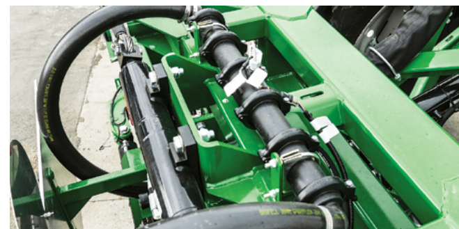
Flow Meter located on top to the boom centre section (shown above).
