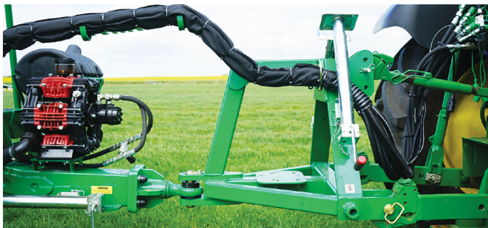
Optional Rowcrop Hitch connected to a tractor with hitch jacks in fold-up away position.
