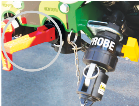
Open the Venturi Valve on the Pressure Manifold.
