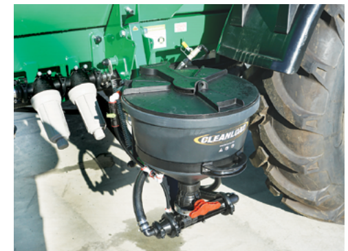
Use the hopper handle to support the hopper, unlock the latch lever, then carefully lower hopper to its working position.
