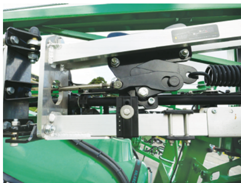
3-Way wing Tip Breakaway mechanism.
