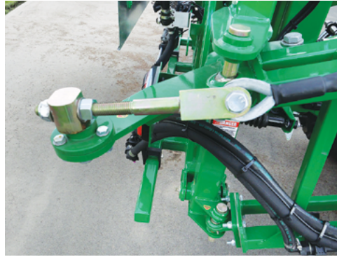
When completed, retighten the locknuts of the cable swivel point adjuster.
