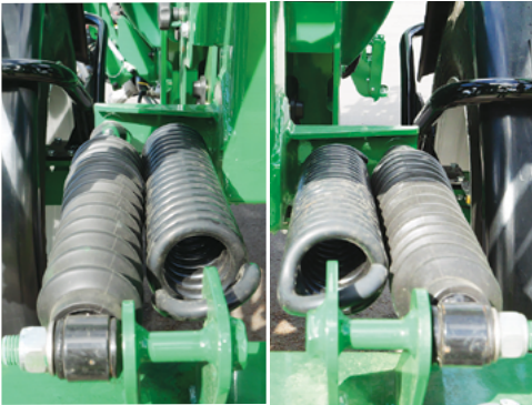
Springs & dampers (on each side of boom centre section) used to align & control Yaw movement.
