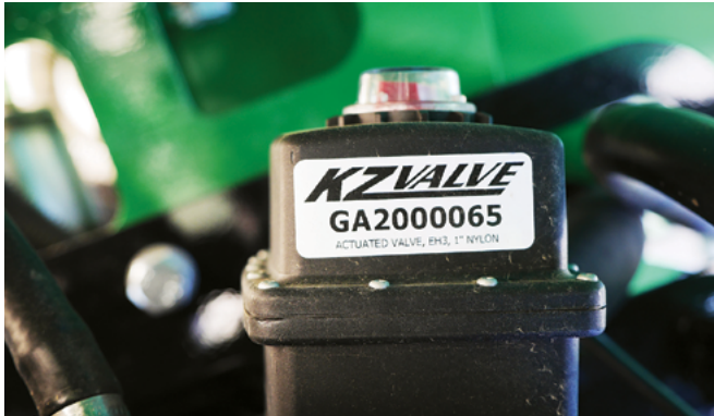
The Boom Flow Regulating Valve should regularly checked & calibrated.
