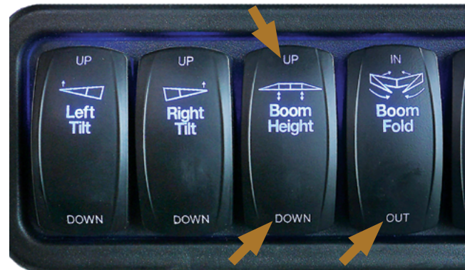
Use the 'Boom Height UP' switch to lift the boom from its rests, then the 'Boom Fold OUT' to unfold the boom, then the 'Boom Height DOWN' to lower the boom.
