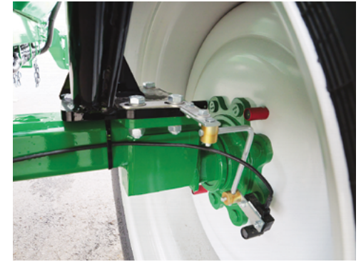
Inspect sprayer axle & wheel magnets.
