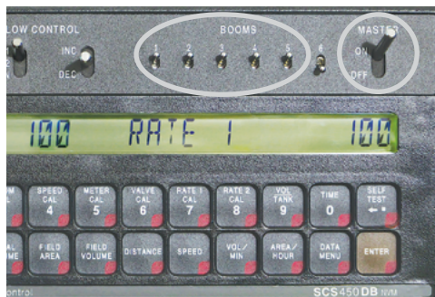
Push On each of the 'BOOMS' section toggle switches, then the 'MASTER' toggle switch to start spraying.
