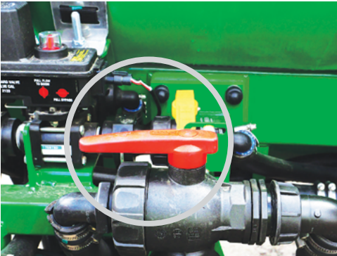
Turn the Three-way Red Handle ball valve (top of the suction filter) to draw liquid from the Main tank (arrow pointing forwards).
