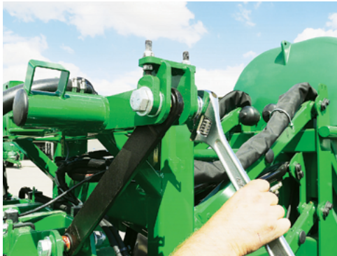
Loosen the bolt & nut clamping the top centre level support (on the centre section side the boom is low).
